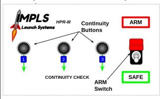
At this time the Arm switch should be set to safe, and the red paddle in the down position to indicate Safe. Distribute your launch leads to the launch pads.
